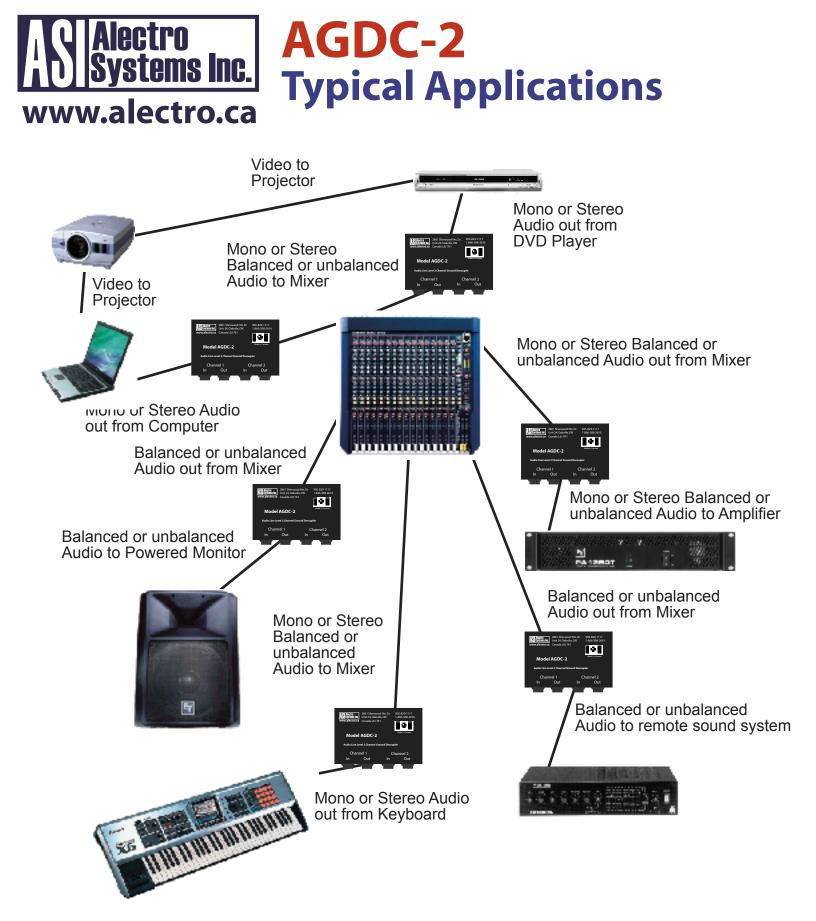
NOTE: All inputs and outputs are Line level, not Microphone level.
