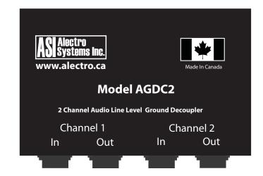
When audio sources are interconnected, sometimes a ground loop is created which causes AC hum. This usually occurs when the devices are connected to equipment in different locations. In order to correct this problem, the grounding on the audio lines needs to be de-coupled.
